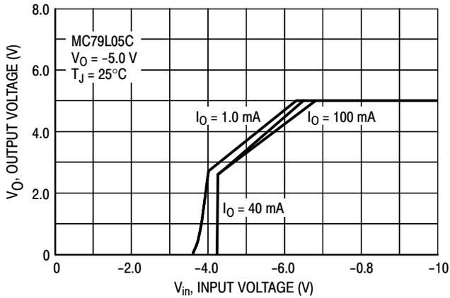
Figure 4. Dropout Characteristics
