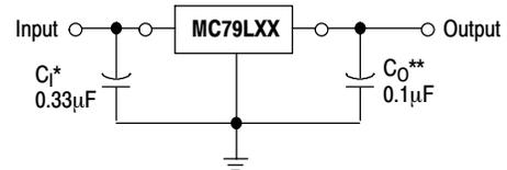
A common ground is required between the input and the output voltages. The input voltage must remain typically 2.0 V above the output voltage even during the low point on the ripple voltage.
